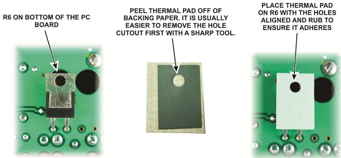
Figure 15. Placing Thermal Pad on R6.
