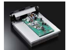
PA unit and heat sink
